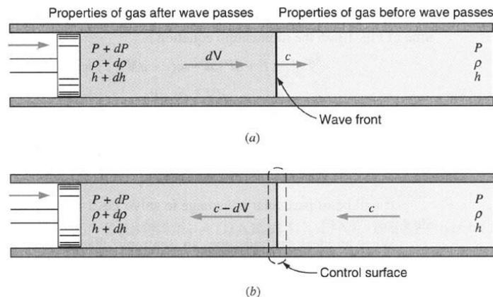
Diagram illustrating sonic velocity. (a) Stationary observer. (b) Observer traveling with wave front.
